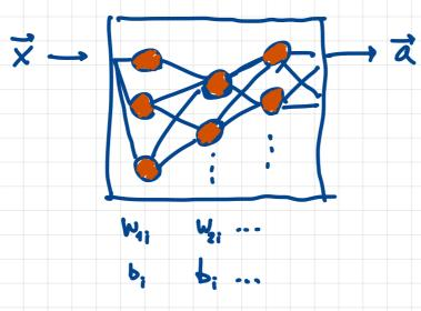
Our job is to aptimize the weights and biases such that the output matches a desired result for a given input.
